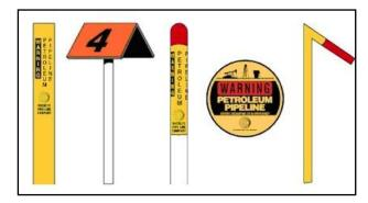
Markers and warning signs only indicate the general location of a pipeline. They cannot be relied upon to indicate the exact position of the pipeline they mark. Also, the pipeline may not follow a straight course between markers. And, while markers are helpful in locating pipelines, they are limited in the information they provide. They provide no information, for example, about the depth or number of pipelines in the vicinity.
